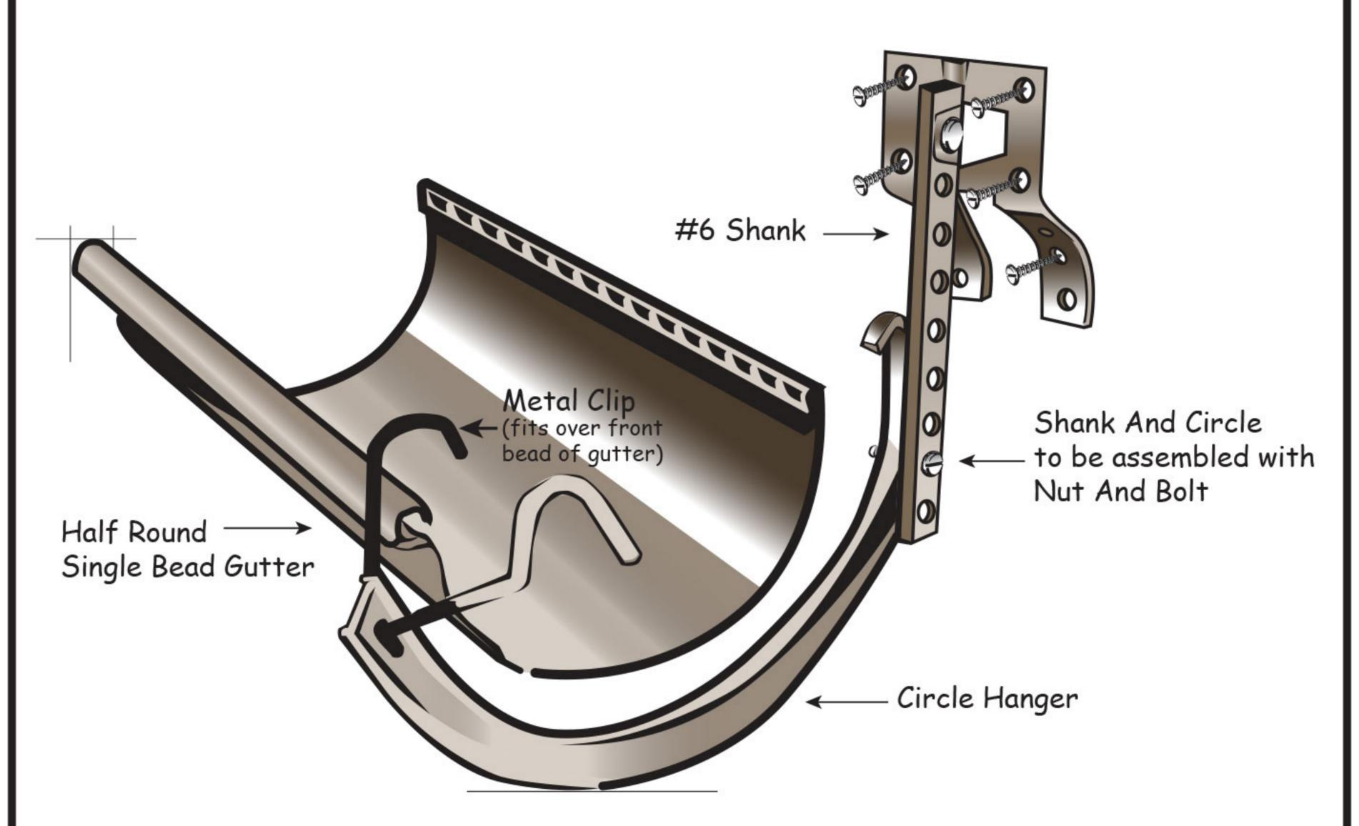
Only one hole on shank and circle will line up for nut and bolt. The flange on the circle hanger will act as a guide to stabilize the two parts together. Position nuts and bolts in lower holes of shanks to provide proper pitch in gutter.
