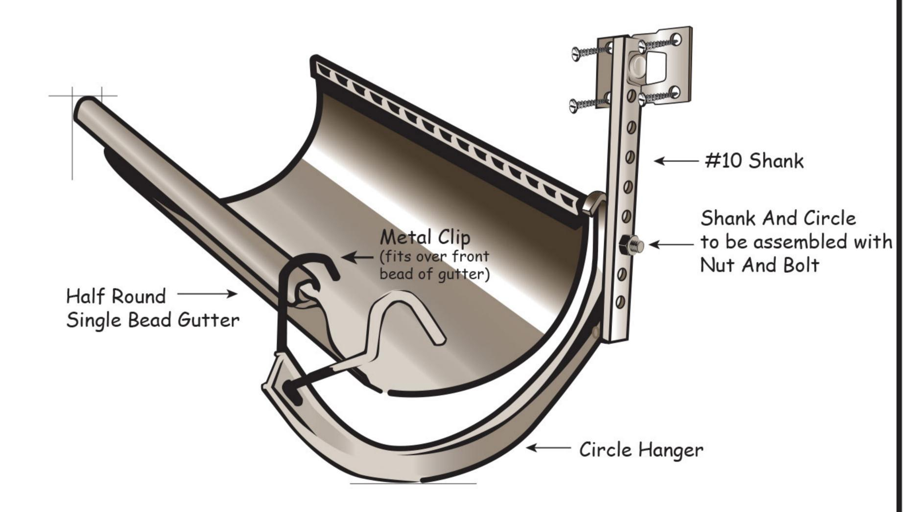
Only one hole on shank and circle will line up for nut and bolt. The flange on the circle hanger will act as a guide to stabilize the two parts together. Position nuts and bolts in lower holes of shanks to provide proper pitch in gutter.
