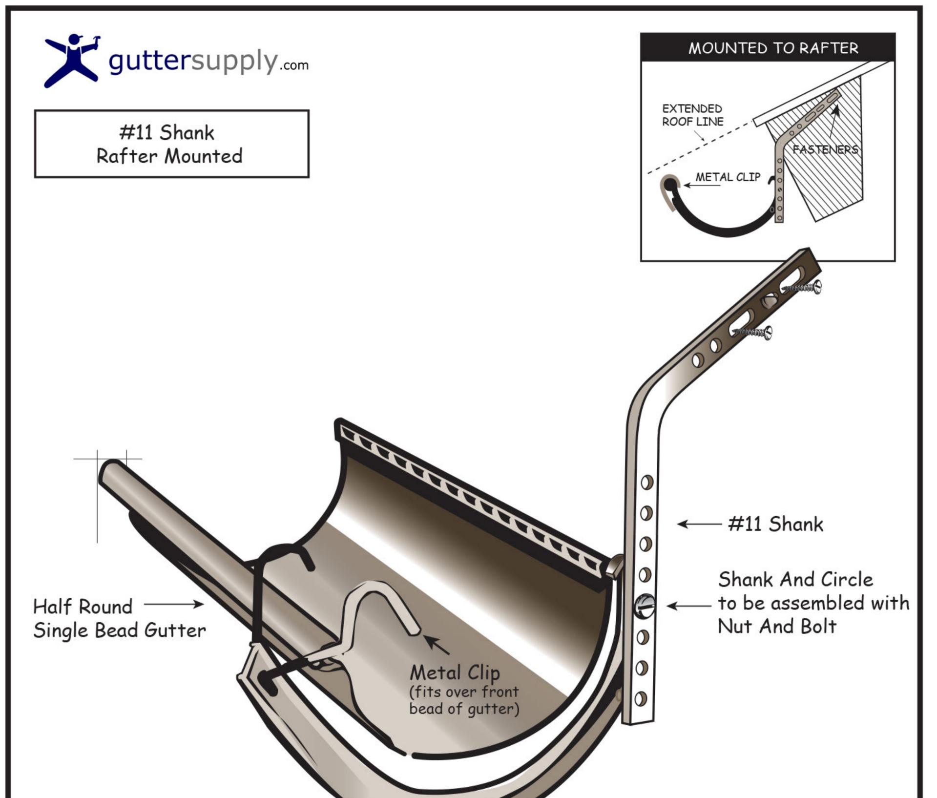
Only one hole on shank and circle will line up for nut and bolt. The flange on the circle hanger will act as a guide to stabilize the two parts together. Position nuts and bolts in lower holes of shanks to provide proper pitch in gutter.
