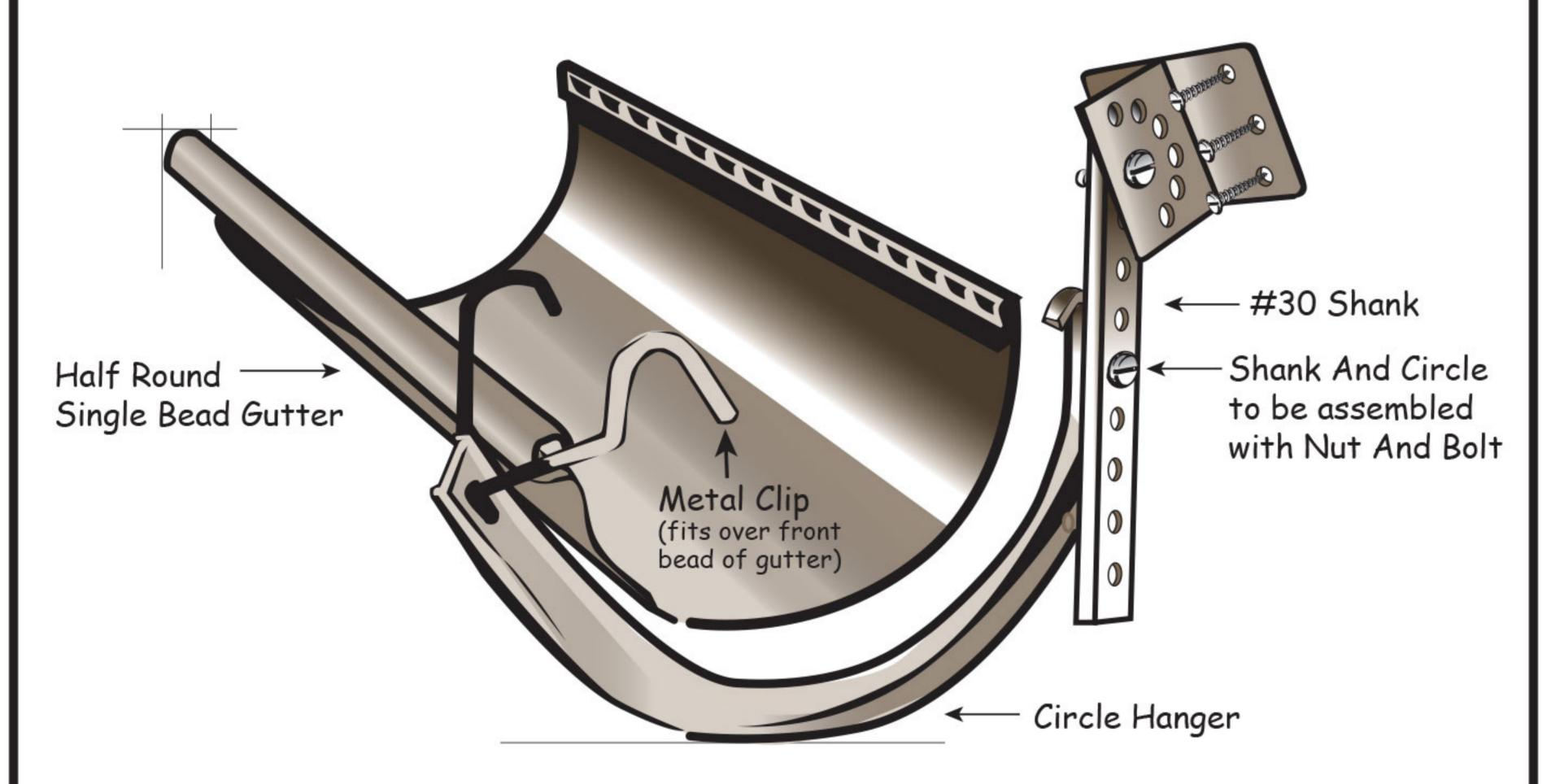
Only one hole on shank and circle will line up for nut and bolt. The flange on the circle hanger will act as a guide to stabilize the two parts together. Position nuts and bolts in lower holes of shanks to provide proper pitch in gutter.
